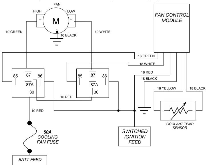
This configuration will activate the low speed input of the fan at lower temperatures, and switches over to the high speed circuit at higher temperatures. It does not allow both fan circuits to be powered at once. This has been specifically designed for Ford two speed fans commonly used for electric fan conversions. **NOTE** Some other two speed fans must have both low and high powered simultaneously, check your fan.
