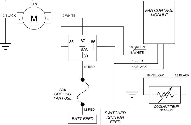
In this configuration, the one fan is run at the lower of the fan on/off points. **NOTE** If using a high power fan, substitute 12AWG wire for 10AWG wire and fuse at 50A or 60A.
